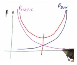
There is an optimal point for the voltage, where there is maximum voltage for minimal leakage.
